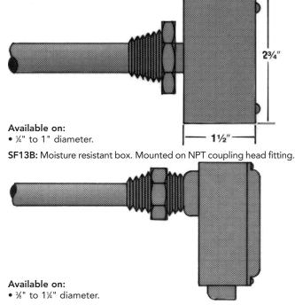
SF13C: Explosion resistant box. Mounted on NPT coupling head fitting.
