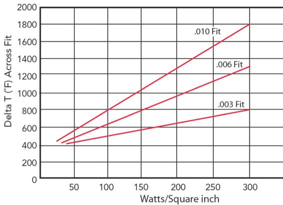
Figure 6: Temperature differential across fit as a function of watt density. Source: Backer Hotwatt
